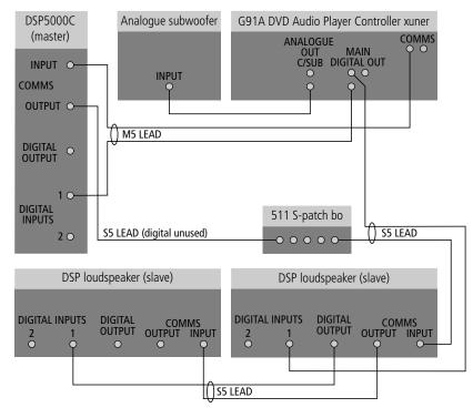
The G91A includes all the digital surround decoding needed to create a 5.1 surround system, directly connected to up to six DSP loudspeakers.
