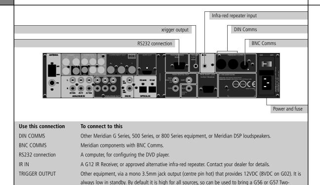
channel Power Amplifier out of standby. Alternatively you can program it to be high for specific sources; eg to
