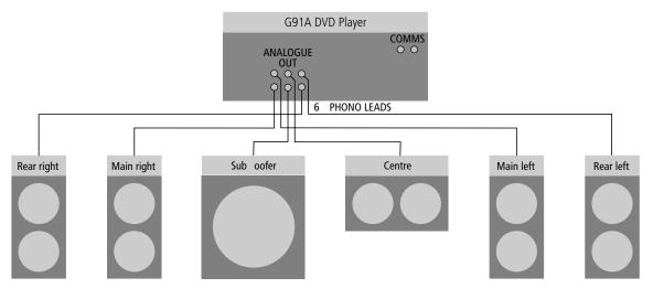
The G91A provides six analogue outputs, and includes surround decoding to allow you to create a 5.1 surround system directly connected to six power amplifiers and passive loudspeakers.
