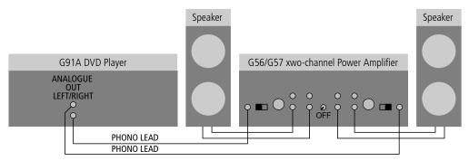
The G91A includes an integrated preamplifier, allowing you to connect it directly to a pair of analogue active loudspeakers, or to analogue passive loudspeakers via a power amplifier such as the G56 or G57.
