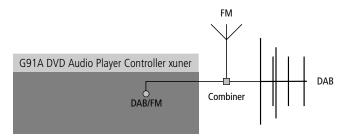
The DAB/FM tuner uses a single antenna input for both DAB and FM reception. For optimum reception we recommend using both DAB and FM antennae with an appropriate combiner.
