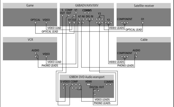
If you are using the G98DH in conjunction with a G68ADV, AXV, or XXV Digital Surround Controller, you can perform video switching in the G68 but take advantage of the video format conversion and scaling in the G98 to drive the display device.
